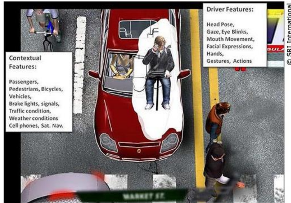
Figure caption 2: Video data include cabin and roadway views. This view illustrates possible relationships between observed driver behavior and the roadway context outside the vehicle, which includes other vehicles, cyclists, pedestrians, and lane markings.
